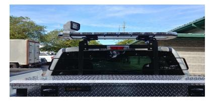
11.12 ONE (1) LED GO LIGHT (Remote Controlled): Model # 20074, Radioray LED. Hard Wired / Mounted to the JV WeCan Series Super LED MODEL JV2A Light Bar. One on PS. No Exposed Wires
