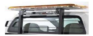
11.12 **TWO (2) LED GO LIGHTS (Remote Controlled):** Model # 20074, Radioray LED. Hard Wired / Mounted to the JV **WeCan Series Super LED** MODEL JV2A Light Bar. One on PS and One on DS. No Exposed Wires
