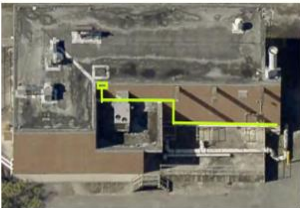
Install new scupper, conductor head and run downspout under AC duct, then down to and adjacent existing drain line.
