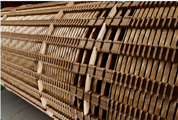
Helical Winding with CTC
