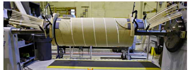
Fully Distributed Regulating Voltage Winding
