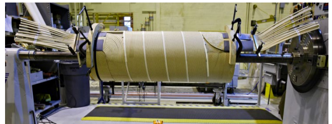
Fully Distributed Regulating Voltage Winding
