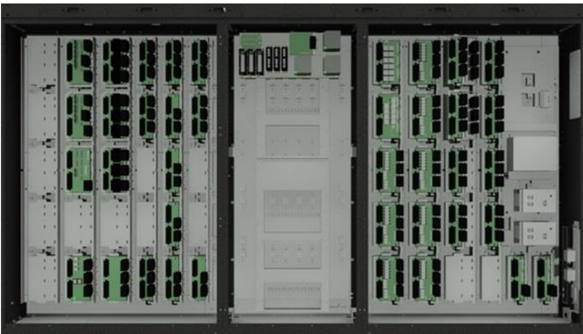
Today's Mark VI Electronic Hardware Structure (Typical TMR)
