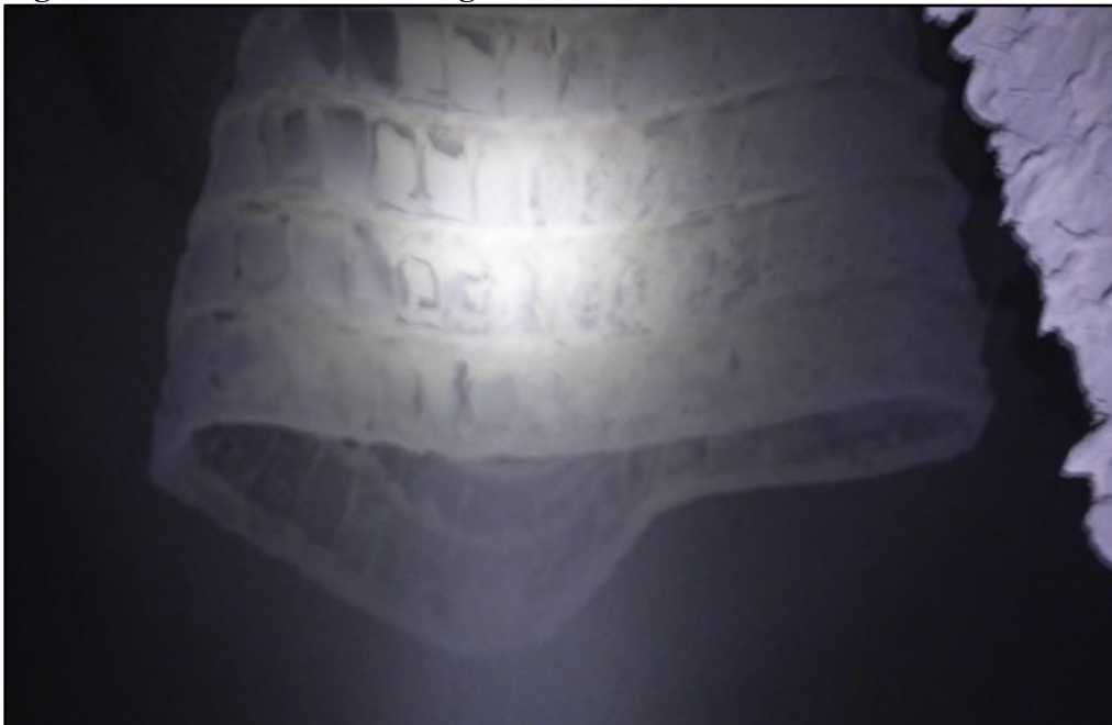
Figure 3. Vortex Finder Damage
